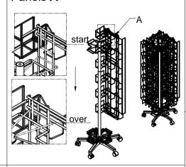
7. Postion 1 wire shelf **B** that is resting on the base up upright **F** into the middle the pole. Place the Pocket Panels just past the middle Hanger Bracket and rest it there temporarily
