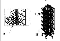
8. Poition the last wire shelf **B** resting on the base, up the upright **F** to just above the bottom hooks of pocket panel **A**. Push wire shelves down, snapping them into place.
